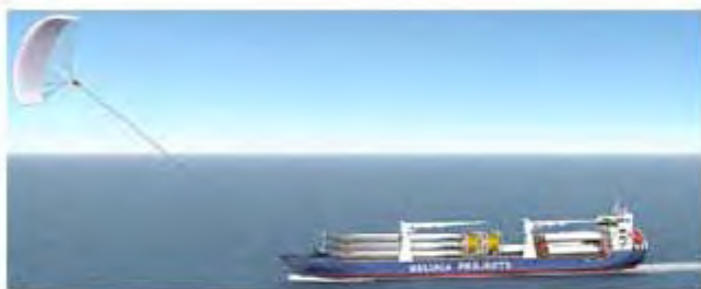
M/V "Beluga Skysail" - operating (System kite)
