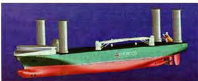
Project "E-1" / ENERCON - under construction (System Flettner-Rotor)
